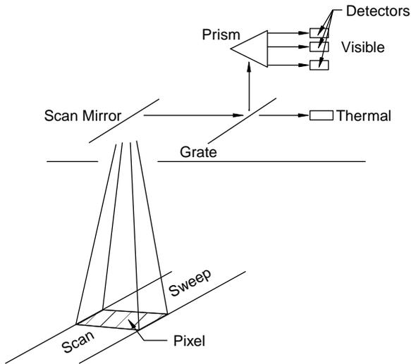
**Figure 15.4** Rudimentary components of an MSS.
