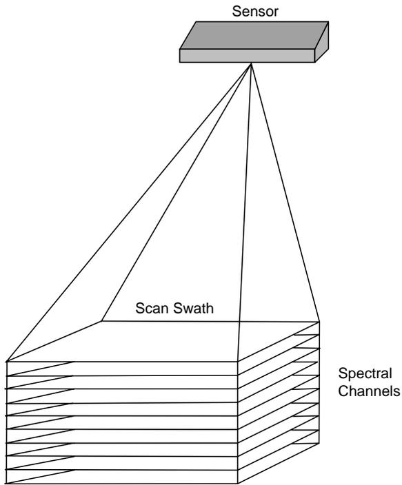
**Figure 15.10** Representation of the concept of a stack of band measurements captured in a single sweep of the scanning mirror.
