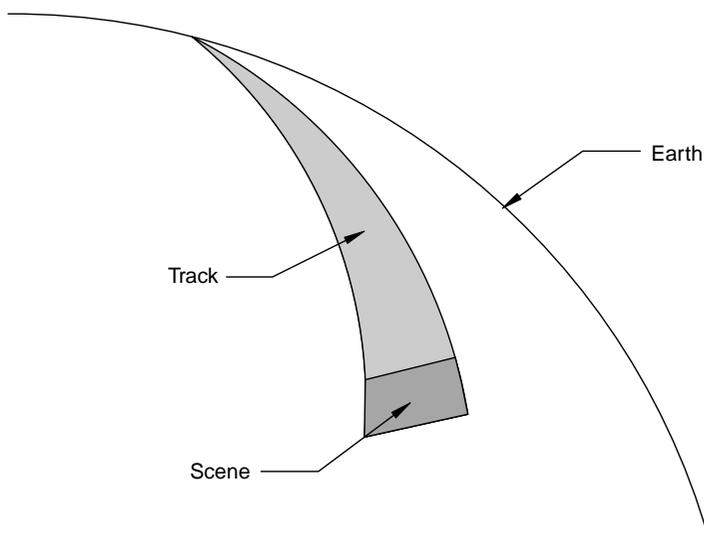
**Figure 15.2** A scene from a scanner's orbital path.
