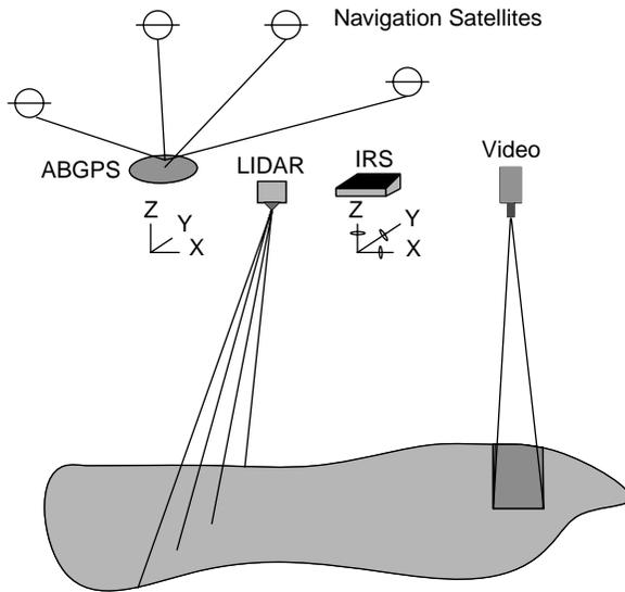
**Figure 15.5** Schematic of the components of an airborne LIDAR system.
