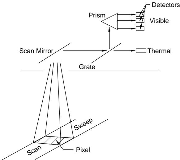
**Figure 15.4** Rudimentary components of an MSS.
