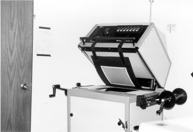
Figure 7.1 An electronic dodging machine used to produce film plates employed in stereo-mapping. (Photo courtesy of authors at Walker and Associates, Fenton, MO.)
