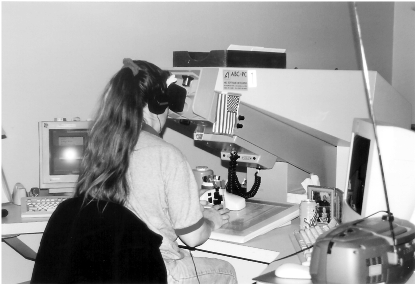
Figure 7.2 An analytical stereoplottter in operation. (Photo courtesy of authors at Walker and Associates, Fenton, MO.)
