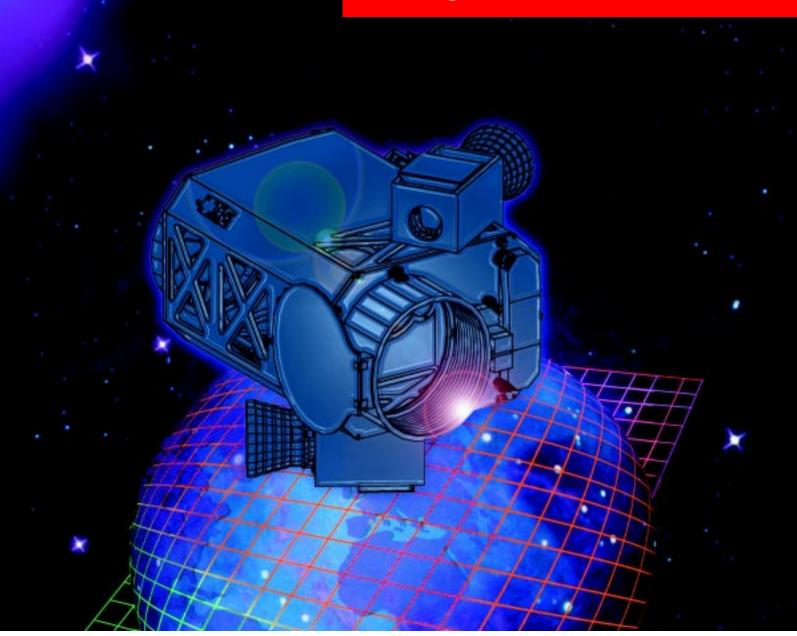
all's High Resolution Camera (BHRC 60) is a state-of-theart optical remote sensing payload that provides simultaneous one-meter class panchromatic and fourmeter class multispectral imagery. This pushbroom implementation is specifically designed to cover broad areas without the need for repointing.
