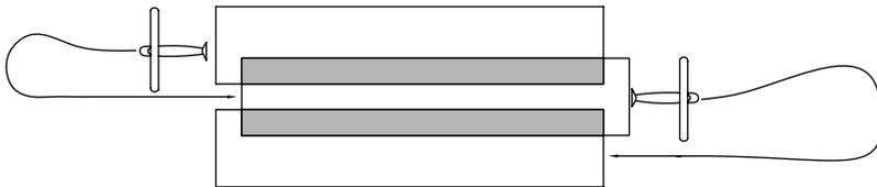
**Figure 6.6** Sidelap on three adjacent flight lines.
