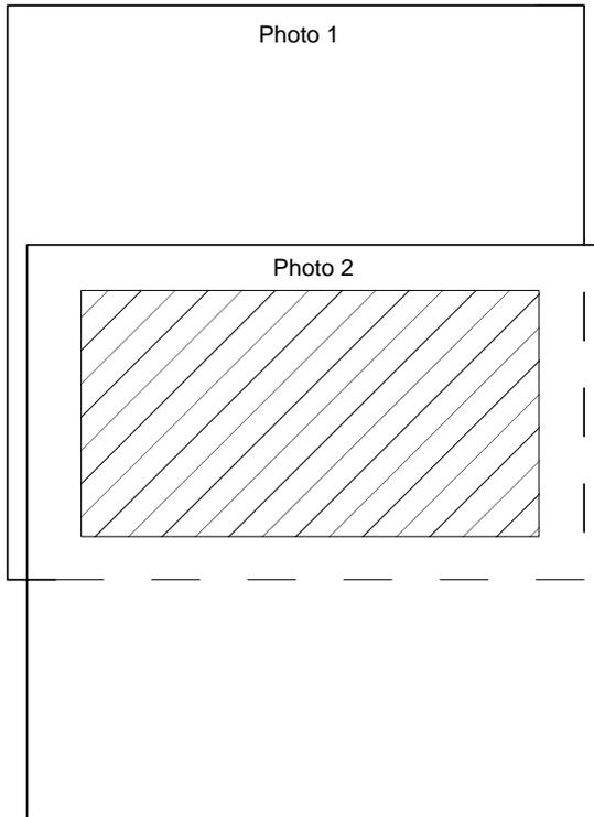
**Figure 6.7** Neat area of a stereomodel.
