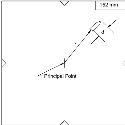
**Figure 6.9** Radial displacement of an image feature.
