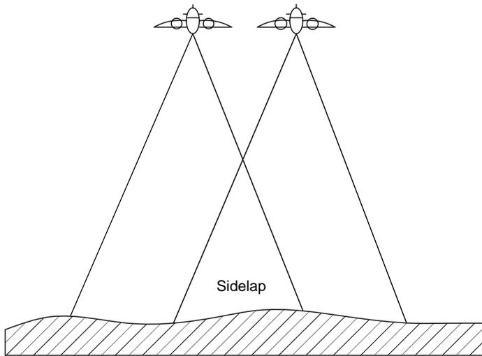
**Figure 6.5** Sidelap between two adjacent flight lines.
