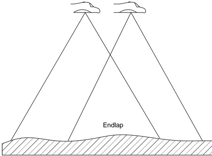
**Figure 6.4** Endlap on two consecutive photos in a flight line.
