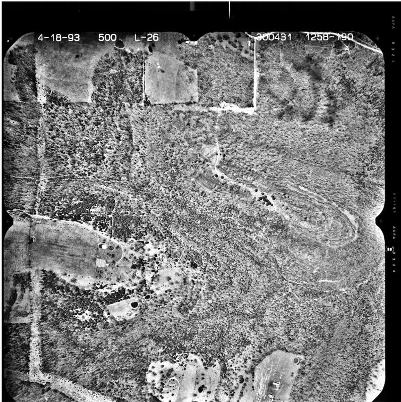
**Figure 6.10** Image displacement on a utility clearing. (Courtesy of Surdex Corporation, Chesterfield, MO.)
